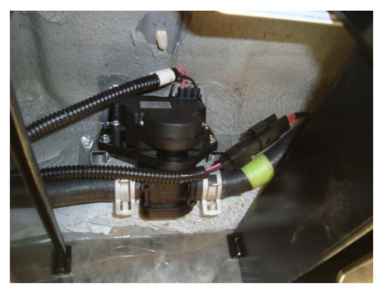
The old valve unit is shown installed in the image above. To begin, disconnect the wire harnesses.
