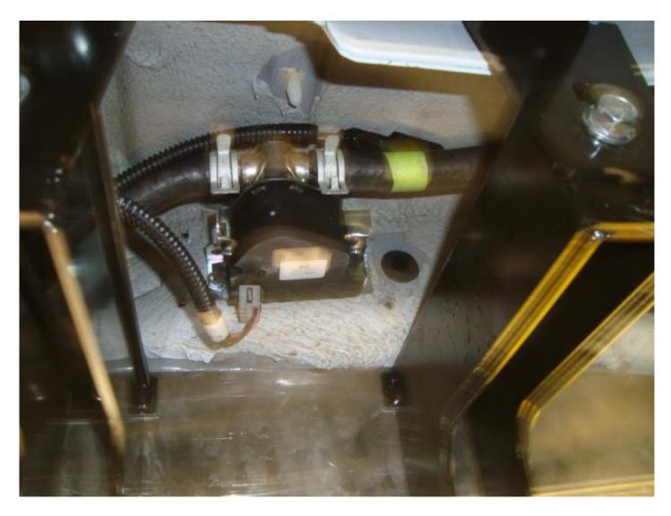
Replace the hoses and clamps and reconnect wire harnesses. The new valve unit is shown installed in the image above.
