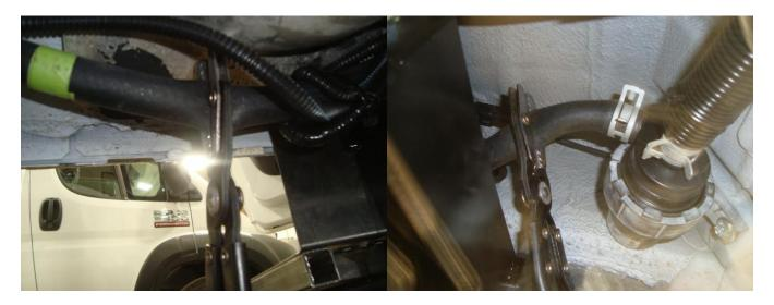
Use the coolant line clamps to clamp the lines on both sides of the unit, as shown above. Then, use the spring clamp tool or pliers to loosen the clamps and back them off of the valve. Use the electric screwdriver to remove the old unit. Then, place and secure the new unit.
