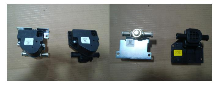
The new unit is shown above on the left. The old unit to be replaced is shown on the right.
