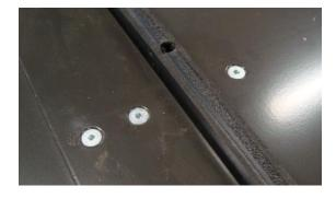
The Base Assembly contains 38 corresponding rivet nuts. If the incorrect rivet nut was installed, there is a possibility that the bolt could extract the rivet nut out of the bottom plate, resulting in a failed connection.
