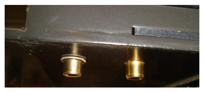
If even just one of these incorrect rivet nuts has occurred on the Base, DO NOT INSTALL THE SHIFT-N-STEP and DO NOT attempt a repair. Contact AbiliTrax Immediately. The defective units MUST BE returned for repair by AbiliTrax ONLY.
