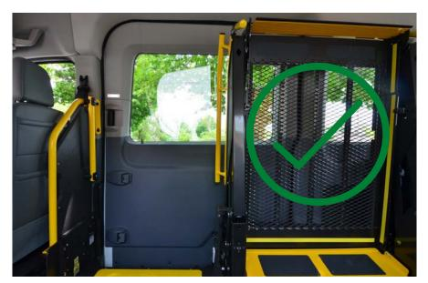
Interlock settings prevent the lift from blocking the doorwary when driving so the potential emergency exit is never blocked
