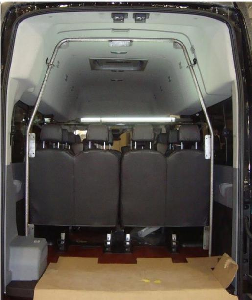
**Step 8** – Temporarily attach the Left and Right Horizontal Support Tubes to the main frame hoop and rear door opening anchor points. This will help establish the position of the mounting feet.
