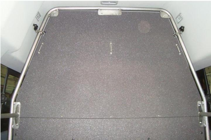
**Step 14** – Re-attach the horizontal support tubes. Tighten the hardware on the upper flange connections first. Tighten the bolts holding the vertical tube lower flange rings to the floor mounting feet. Tighten the bolts securing the upper angle brackets thru the headliner spacer tubes next. Finally, tighten all remaining bolts.
