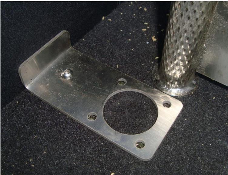
Place the round flange ring back into the foot and install a "horseshoe" clamp plate and the remaining 4 screws. Do not yet fully tighten any of the hardware.
