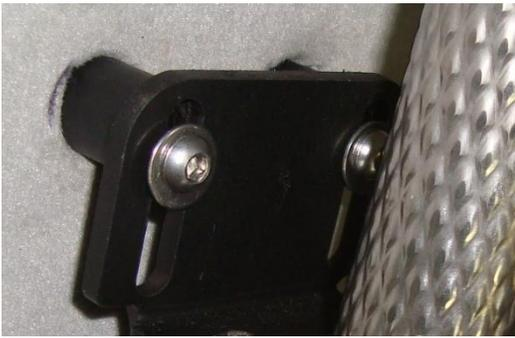
**Step 6** – Assemble the main frame hoop (2 identical vertical tubes and a horizontal tube) by butting the ends together at the flange rings while simultaneously positioning the flange rings into the large hole in the angle brackets. Place a “Horseshoe” clamp on each side of the bracket and install the button head bolts and flange nuts. Leave hardware loose.
