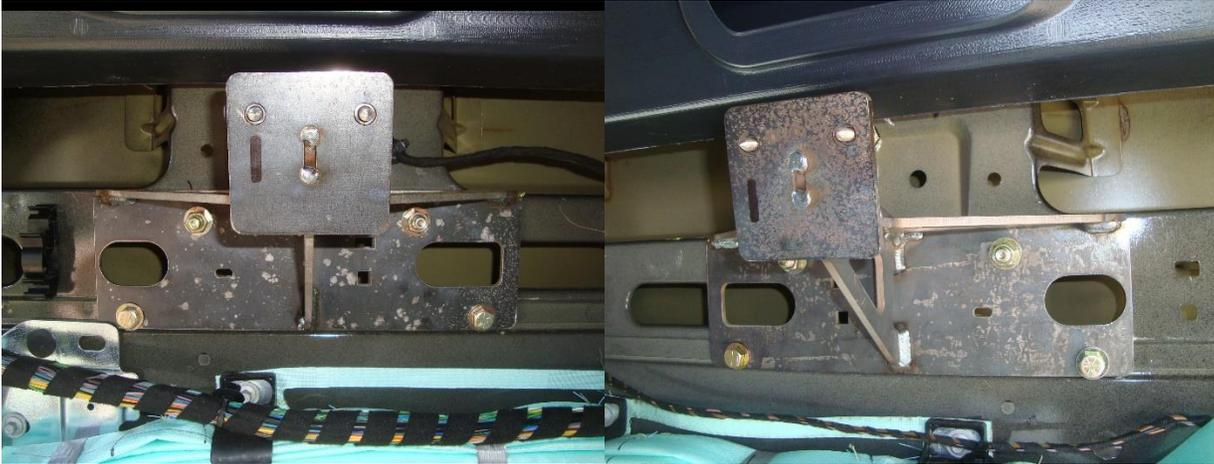
**Step 3** – Temporarily clamp the brackets in place and mark the hole locations. Remove the brackets and drill 4, 13/32" Dia. Holes for each bracket. Reinstall the brackets using 3/8" Hardware and re-secure and protect all wiring.
