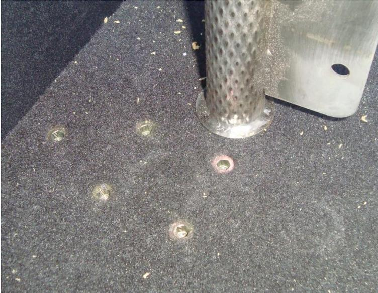
Attach foot to floor using only the single hole location.
